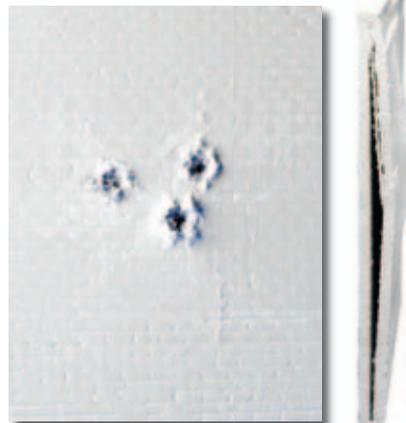
*The ply delamination process of energy absorption is illustrated in the photo to the left. Three .44 magnum bullets are totally encapsulated by the fiberglass panel to meet UL 752 Level 3 and NIJ Level 3A specifications.*
